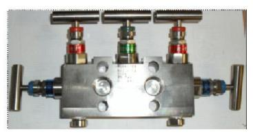
Direct style block mounted five-valve manifold, instrument mount to pipe connection. Offering two isolation valves, two vent valves and one equalizing valve. Used in differential pressure transmitters and static instrument applications. Standard 2 x 1/2" inlet x direct mount (54mm centres) with 2 x 1/4" vent port.
